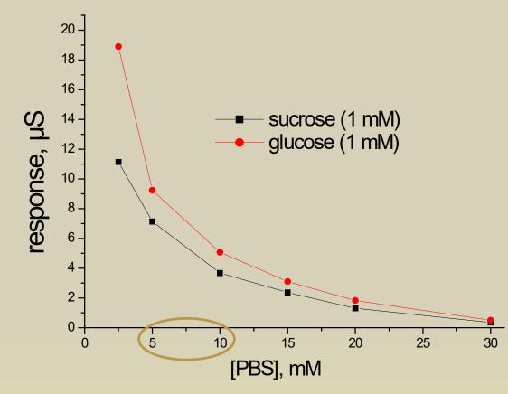
Dependences of biosensors responses on buffer concentration. Measurement were carried out in phosphate buffer, pH 6,0.
