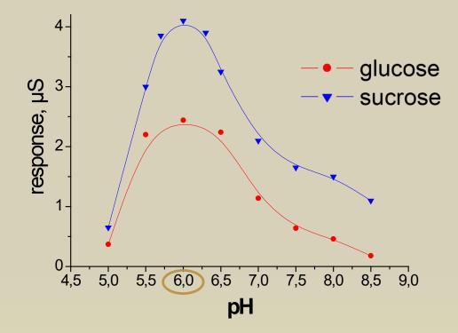
Concentration of substrate was 0.5 mM. Measurement in polymix buffer solution
